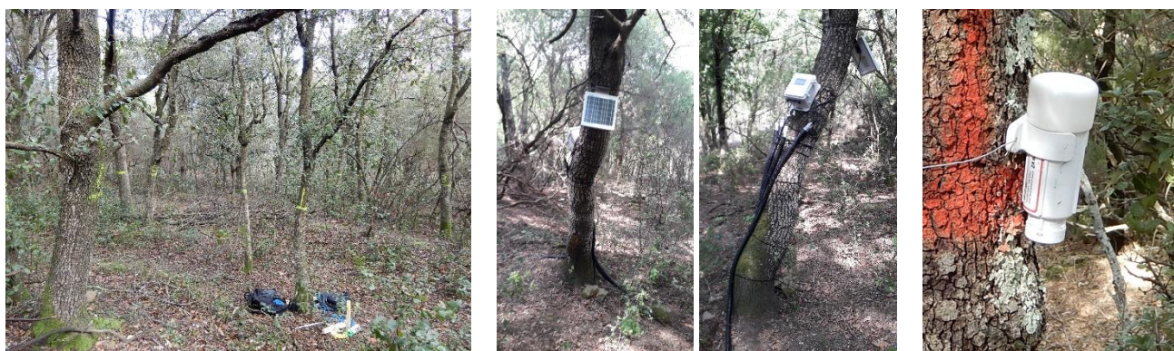
Figure 10. Installed monitoring network: left, forest inventory plot; centre, dataloggers and soil moisture sensors; right, air temperature and relative humidity sensors.
